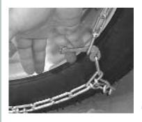
Next fasten the outside fastener making sure it is as tight as possible. Drive a short distance and re-tighten all fasteners. For best results, make sure all connections are equal and as tight as possible.
