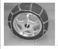
Drape the chain over the tire, again making sure the cross chain hooks are facing upward. Hooks that face down (towards the tire) will cause damage to the tire.
