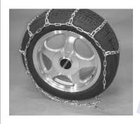
Pull one cross chain down to the point where the tire meets the ground. Move the vehicle so that 1 or 2 cross chains pass under the tire.
