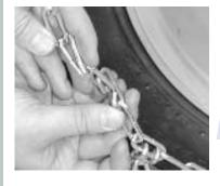
Reach behind the tire and fasten the inside connector on the 2nd or 3rd link.
