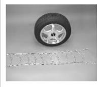
Park vehicle on firm level ground, and turn off the engine. Set the parking brake. Unroll the chains and lay them out flat making sure there are no twists or tangles. Make sure the smooth side of the cross chain hooks are toward the tire.
