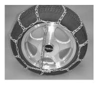
Attach the rubber tensioner to take up the additional slack. To make this simpler, attach the first hook at the "11 o'clock" position, the next at the "5 o'clock" position and so forth. Tighteners must be purchased separately.
