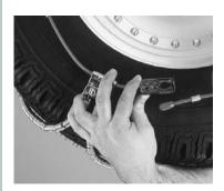
Take the bushing end of the lower fastener and thread it through the lower keyhole (the one near the ground), using the same process as the top fastener. Please refer to the following page for a detailed look at making this connection
