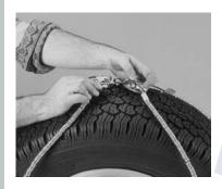
Reach around each side of the tire and grasp both ends of the non-split cable (the cable that is furthest away from you). Pull both ends to the top of the tire so the fasteners can be seen and manipulated more easily. Fasten the curved "C" hook through the fastener hole.
