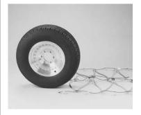
Park vehicle on firm level ground, away from traffic and turn off the engine. Set the emergency brake. Remove any wheel covers. Chains should be installed on drive tires. Lay the cable chain on the ground with the smooth side (TIRE SIDE) of the cross member connection up.
