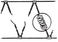
[A] Fragmented traction coils - Traction coils in middle of cross members begin to fragment due to speeds over 30 mph and/or excessive bare pavement driving.
