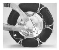
Attach the rubber tensioner to take up the additional slack. To make this simpler, attach the first hook at the "11 o'clock" position, the next at the "5 o'clock" position and so forth. The open side of the hooks must face away from the tire. No further adjustment is necessary.
