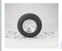
Move the chain in a sweeping motion under the vehicle so the open mid-section is positioned up against the backside of the tire. This sweeping motion can best be done while kneeling in front of the tire.
