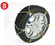
This is how a properly installed chain should appear on your tire. Your vehicle may now be driven without further adjustment.
