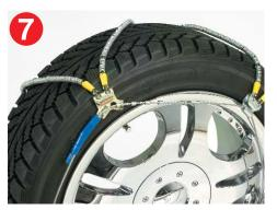
To secure the free ends of the cable, slide the plastic spirals over them with a twisting motion. If insufficient cable is available for plastic spirals to secure, "tuck" the short end up next to the crossmember anchor points, as shown here.
